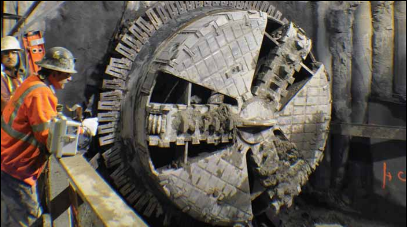
The Robbins EPB TBM broke through on November 21, 2009 with record advance rates of up to 210 m (690 ft) per week.
