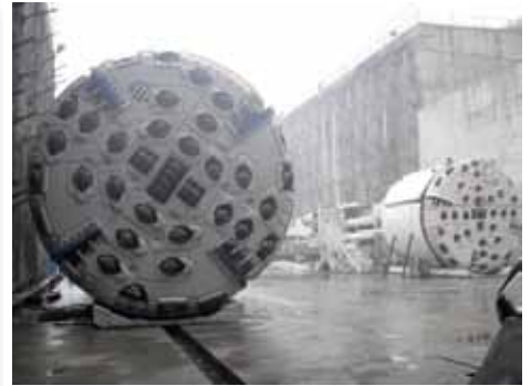
Left: Onsite assembly of major components for the Mexico City Metro's EPB was completed in about eight weeks.
